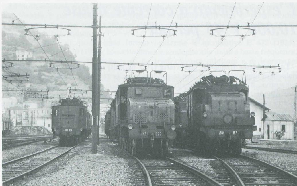
Fig.26 - Locomotive Gr. E.333, E.431 ed E.554
